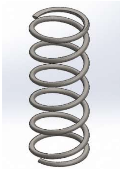
Figure 2: Modeling of helical coil spring (SAE 9254)
