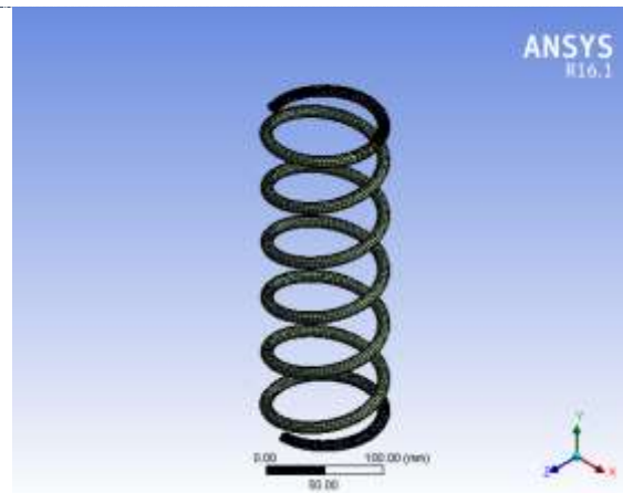
Figure 4: Meshing of coil spring (SAE 9254)
